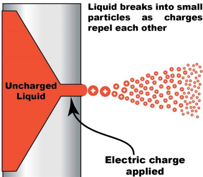
This concept is combined with the process of atomization. By applying an electrostatic charge to the liquid, each particle becomes charged with the same positive charge. Again using the basic principle that opposites attract and similar charges repel, the particles are naturally repelled by one another, and freely break apart or atomize. This is the primary concept that allows for a more even coating.
