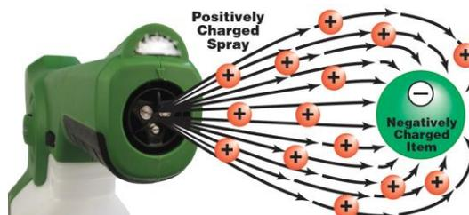
**The benefits of using electrostatic sprayers in the cleaning industry:** The most important benefit of electrostatic sprayers in the cleaning industry is around the application of disinfectants and sanitizers.
