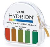
Quat test strips can be used to check the quat ppm level when used in sink basin cleaning, part number 421200.
